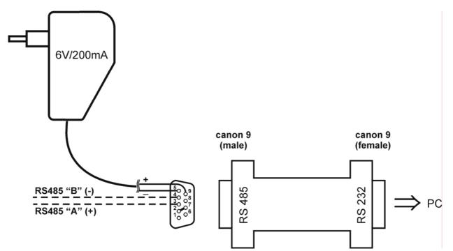
The ELO E06D converter is an optional accessory for connection of transducer/transducers with RS485 interface to the PC via serial port RS232. Connect connector marked RS232 directly to the PC, connect power to connector marked RS485. Power voltage +6V DC from an external acdc adapter connect to pin 9, 0V connect to pin 5. Also mutually connect pin 2 and pin 7. Link RS485 is connected across pin 3 (A+) and pin 4 (B-).
